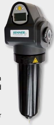
RENNER compressed air filters are suitable for separating oil and water aerosols as well for the removal of solid contaminants from compressed air. Even dust is securely kept on the surface and in the filter material. A filtration efficiency of almost 100 percent is reached through the use of various filtration mechanisms, such as separation by direct trapping, inertial impact and Brownian motion.
